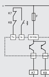
In order to function correctly, any modules or PLCs connected to the OSx safety electronic outputs must be able to withstand cyclical deactivation tests performed on the same.
