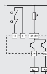
Feedback circuit for external contactors with manual or monitored start
