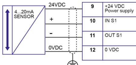
**3 WIRES CURRENT SENSOR WITH EXTERNAL POWER SUPPLY**
