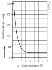
Safe breaking, no continuous arcing under the curve, max. 1 switching cycle/s
