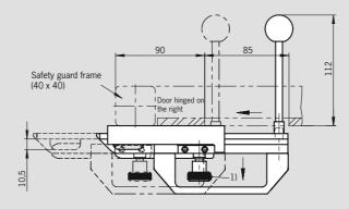
Bolt with detent mechanism (only for bolts with escape release): latches in open position and prevents unintentional closing of the bolt. Unlocked by pulling the detent knob upward.
