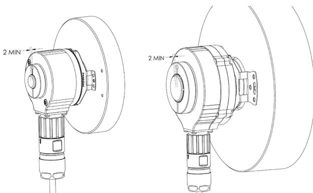
For safe clamping verify the driving shaft extends at least 2 mm out of the encoder. Check the position of the stator coupling. Avoid compressing or extending it to insure a minimal load on the bearing block.
