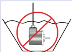
Do not dip encoder into water, check encoder's IP code.
