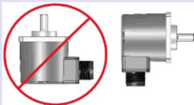
Avoid installing with shaft upright, liquid may pool and eventually cause internal leaking.
