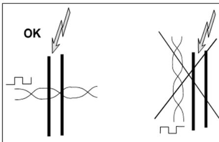
**Power supply wires cross section**
