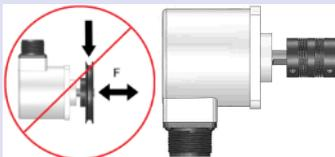
Do not hard couple encoder to driving shaft. Instead use flexible couplings to minimize stress on encoder bearings.
