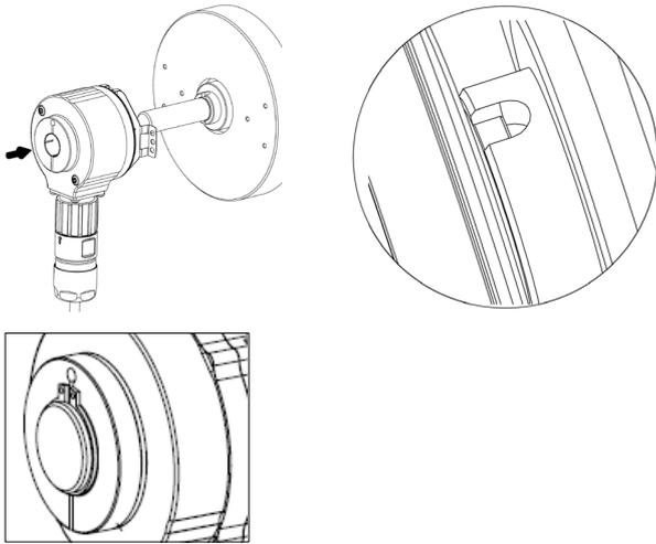
Check that the positive locks are in the correct position for proper engagement.
