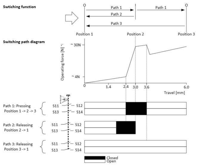
\*)The operating force will change by using rubber boot and depends on the operating temperature.
