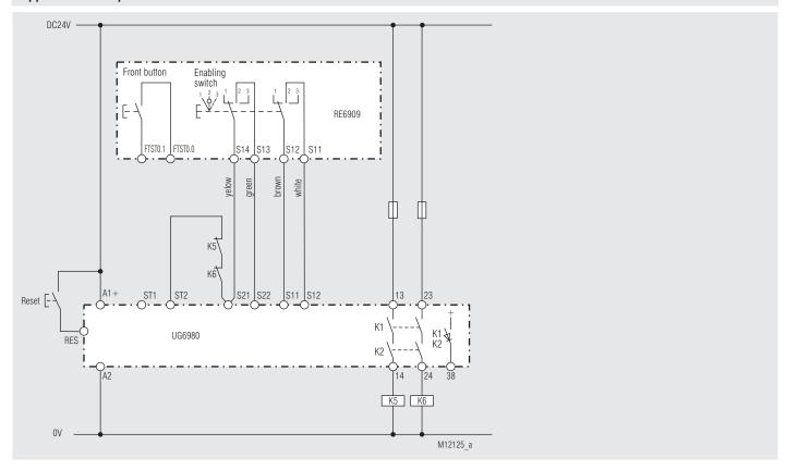
The multifunctional safety module UG 6980 is configured via a selector switch and must detect cross-faults in the supply line of the enabling switch in its configuration.
